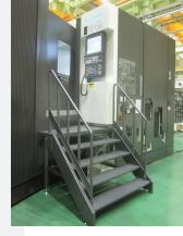
CNC panel swivels out for easy access and folds flat to save space. A manual pulse generator simplifies work set-up and precise positioning. (Shown with optional steps)
